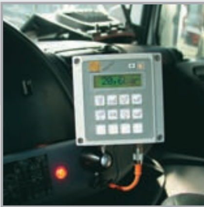
The option of operating the mixer from the driver's cab is a standard feature, while the configuration varies depending on the pump system
