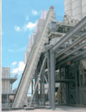
Different lengths of the elevator track (skip) are possible.
