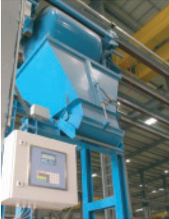
The specific requirement indication point allows different concrete types and quantities to be requested directly during production.
