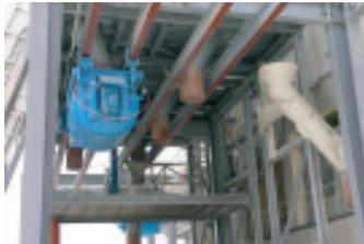
Example of three mixing systems featuring six discharge points for the bucket transport system. Right: Extension chute for loading of the truck mixer.
