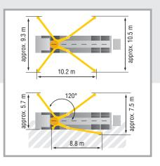
Country-specific admission requirements for 4 or 5 axles must be checked. Dimensions are model-dependent and may vary. Gross weight depending on equipment and chassis  $\leq$  40 t
